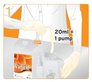
Using the Vacucid® Systematic, dilute at 2% (40ml for 2 litres of solution).
