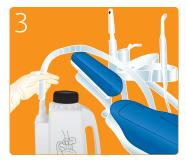
Attach the Vacucid® Systematic to the suction system and aspirate the diluted solution.
