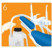
Flush by sucking the clean water through the system (minimum 1 litre).
